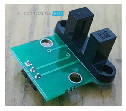
Coming to control unit, it is made up of LM393 Voltage Comparator and a few passive <u>electronic components</u>. The signal from the photo transistor is given to the LM393 and based on the presence or absence of an object between the Infrared LED and the Photo Transistor, the Output of the LM393 IC will either be HIGH or LOW.
